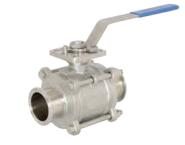
**BV2C ball valve** is manufactured of CF8M (316) stainless steel. It is a three piece **encapsulated** valve with clamp ends and ISO 5211 mounting pad.
