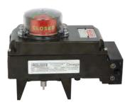
The S- series combines a compact enclosure with limit switches, visual indication and integral solenoids for position indication plus valve actuator control and 3-position control for Bradford 3-way ball valves and 180 degree actuators. NAMUR proximity switch options and EEx is solenoid valve also make the S-series suitable for use in intrinsically safe applications.
