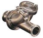
**Y-ball check valves** are used where full flow and low pressure drop of product during processing is required. When the flow of product stops, the PTFE ball rolls back and seats, thus preventing backflow. The Bradford<sup>TM</sup> two-piece body design is available in  $1\frac{1}{2}$ " - 3" sizes.
