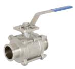
**BV2L** and **BV2M** ball valves are characterized V Seat 2-Way CF8M (316) sanitary stainless steel control valves. It is a three piece encapsulated valve with clamps end and ISO 5211 mounting pad.
