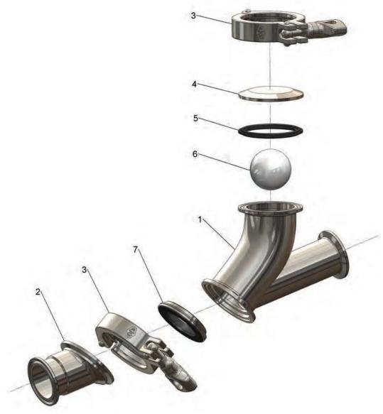
EPDM Seal Kit contains: #5 (1) EPDM end cap gasket #7 (1) EPDM/CF3M seat
