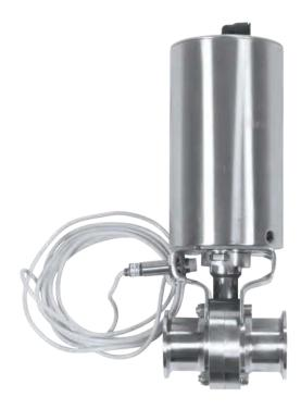
**B5101** series butterfly valve with vertical canister air to open, spring to close actuator. Normally closed, 10-30VDC, 3-wire PNP proximity sensors
