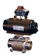
Bradford<sup>™</sup> automated 2-way encapsulated ball valve with spring return fail close actuator and NEMA 4/4X limit switch with two SPDT mechanical switches.
