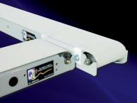
The 90° Transfer Plate covers the gap between perpendicular conveyors, easing product transfer. They are not intended for high friction or cleated belts. The discharge conveyor must be pushing. The customer must drill screw holes to mount plate.
