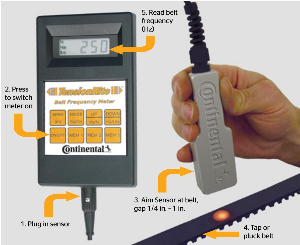
Following these simple steps will allow you to measure the vibration frequency of the belt. This value is independent of span or mass values but is very useful as an index for belt system maintenance, sometimes the only number you will need. For example, the MaximizerPro™ drive analysis program gives tensioning targets in Hz as well as in force units (newtons and pounds-force).
