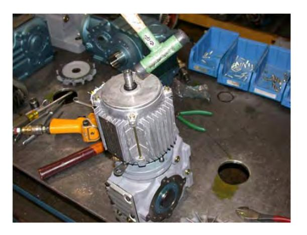
Install the fan using gentle taps with the dead blow hammer.
