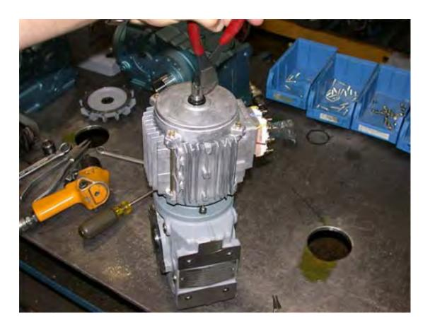
Remove the rubber v-ring from the rotor shaft.
