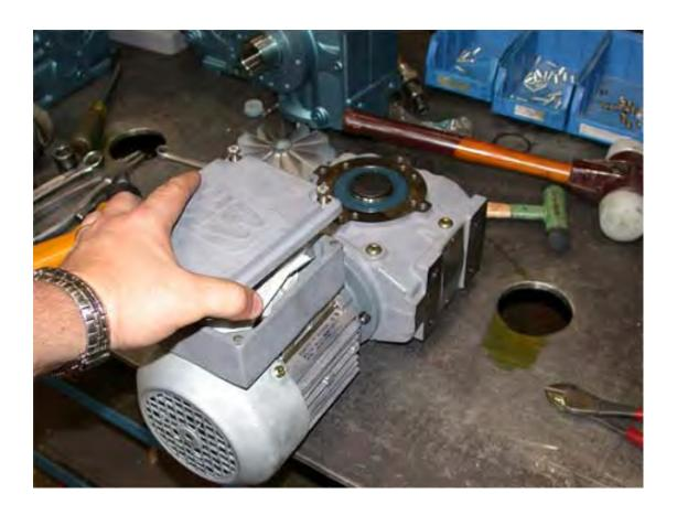
Reconnect power and confirm the proper operation of the motor and attached equipment.
