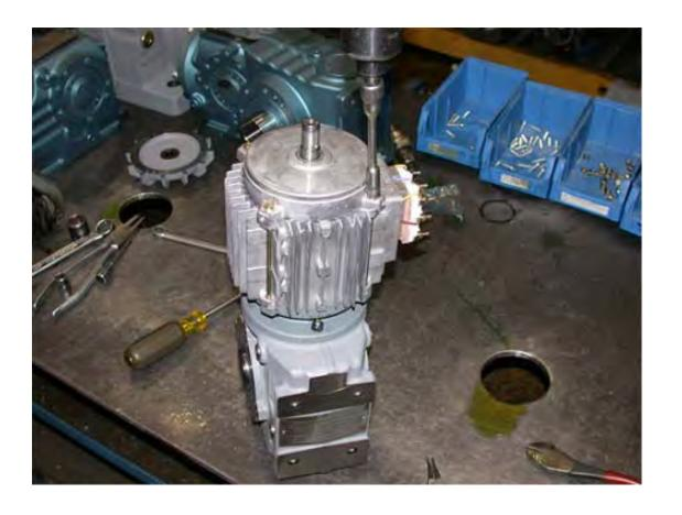
Place the medium-sized flat-tip screwdriver between the stator and the motor end bell. Gently pry the stator at several locations to loosen it. Use caution to avoid damaging the stator fins!
