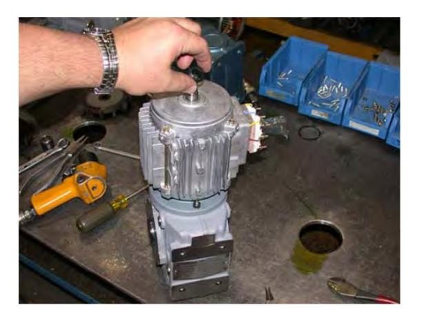
Using the appropriate metric socket, remove the four (4) motor tension rods.
