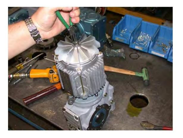
Place the fan guard over the fan, lining up the fan guard holes with the holes in the end shield.
