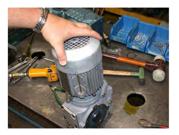
Using the appropriate metric socket and driver, install the four (4) fan screws.
