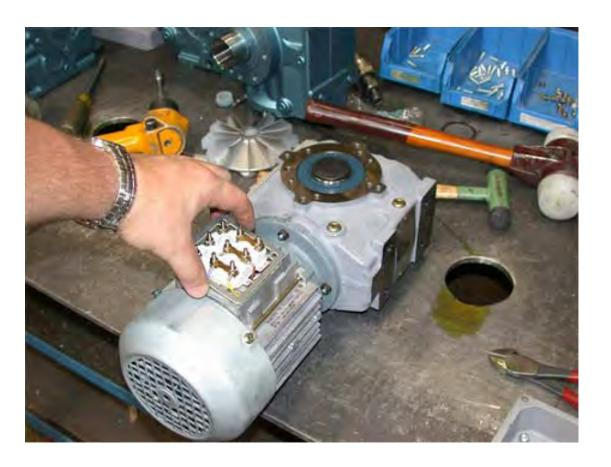
• Using the four (4) Torx screws and Torx driver, install the conduit box into its previous location to ensure that any drain holes remain in their proper position.
