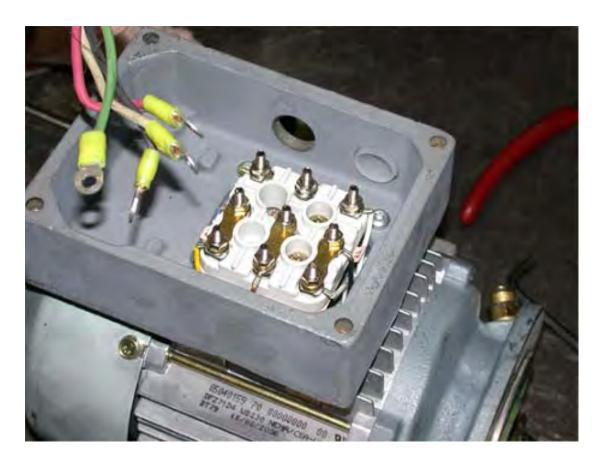
Remove the four (4) Torx screws inside the conduit box.
