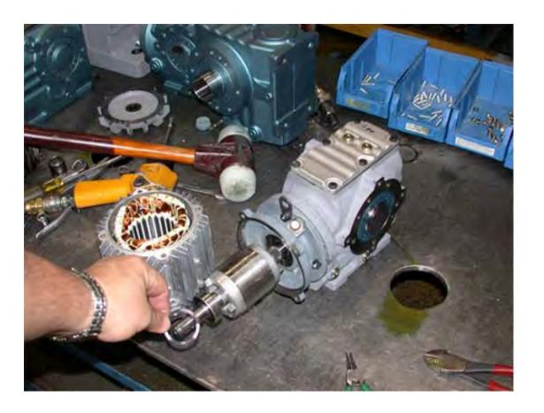
Tap the inside of the motor end shield to gently remove it from the stator.
