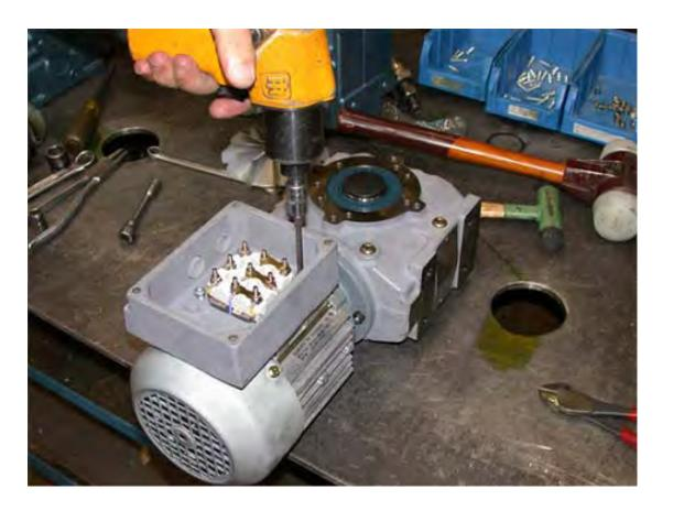
Reconnect all of the wires according to the appropriate wiring diagram.
