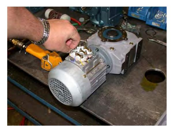
Using a metric nut-driver, remove the 4 small screws that hold the fan guard in place.
