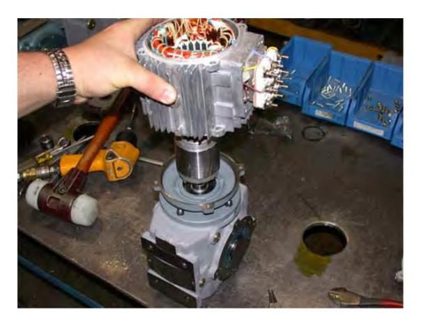
• Line up the tension rod holes. Then, gently tap the stator onto the flange.
