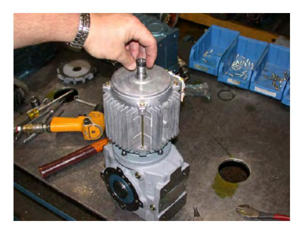
Install the A-key using the dead blow hammer.
