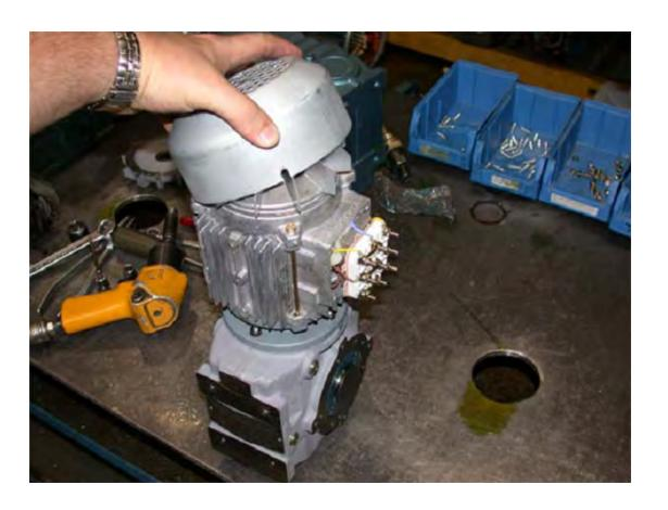
Using the external snapring pliers, remove the snapring that secures the fan.
