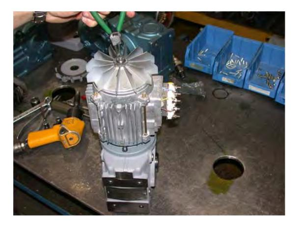
With the medium-sized flat-tip screwdriver, gently pry the fan up and down to loosen and remove it. Use caution to avoid damaging the fan!
