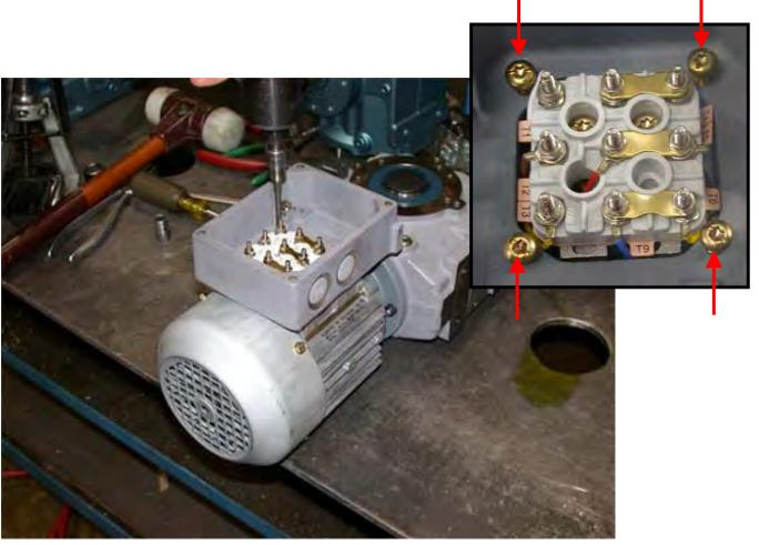
Remove the conduit box from the motor.
