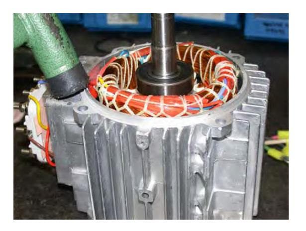
Slide the wavy washer onto the rotor end.
