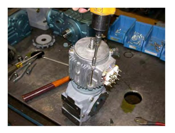
• Lubricate the rubber v-ring with oil or grease. Slide it over the end of the rotor shaft until it seats firmly against the motor end shield.
