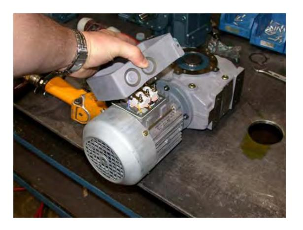
Remove the conduit box gasket from the motor.
