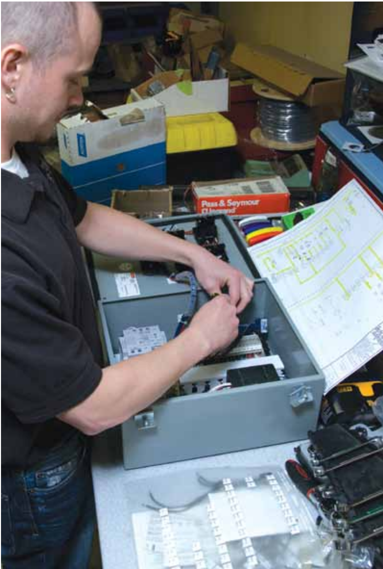
A Creswell Richardson technician is shown here assembling a control box before delivery to a customer.
