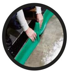
Place the widest side of Spill Berm down for the best seal
