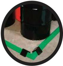
Clear away any debris from the area where the Spill Berm will make contact with the floor.
