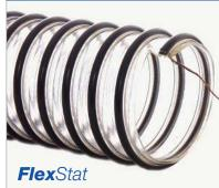
**Construction:** Specially formulated static dissipative polyurethane hose reinforced with a rigid ABS helix and an embedded copper grounding wire.
