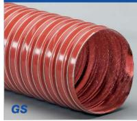
Construction: Double-ply silicone coated fiberglass fabric hose reinforced with a spring steel wire helix & external filament fiberglass cord.
