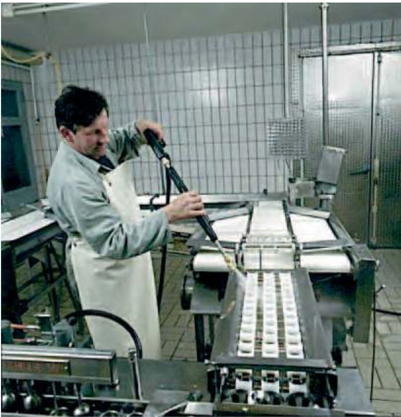
Low pressure cleaning of food conveyor belts
