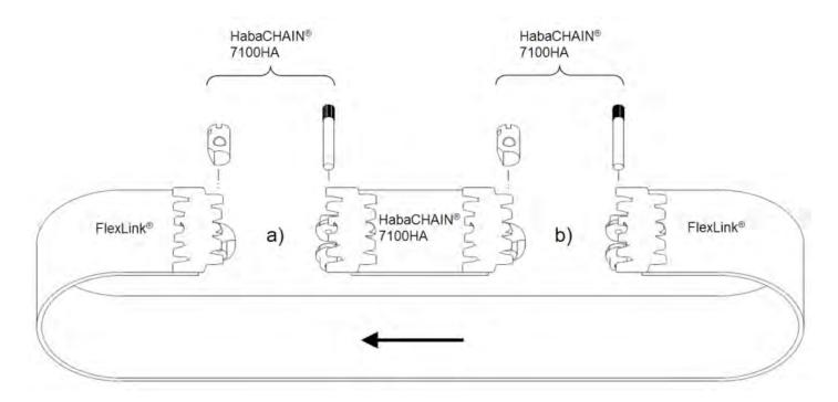
a) + b) Use the HabaCHAIN<sup>®</sup> C7100K0248--HA bushing and the knurled pin to connect the FlexLink<sup>®</sup> chain section with the HabaCHAIN<sup>®</sup> C7100K0248--HA chain section and vice versa.
