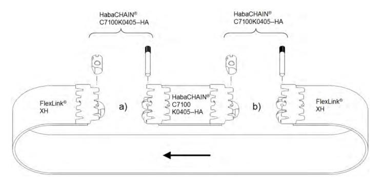
a) + b) Use the HabaCHAIN<sup>®</sup> C7100K0405--HA bushing and the knurled pin to connect the FlexLink<sup>®</sup> chain section with the HabaCHAIN<sup>®</sup> C7100K0405--HA chain section and vice versa.
