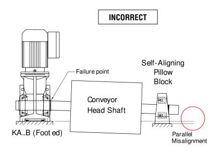
**Problem:** Even though a self-aligning bearing is used, the parallel offset caused by different mounting planes creates a bent conveyor shaft and a bending moment (i.e. an overhung load) at the edge of the reducer. The result of this overhung load is either premature failure of the reducer bearings or fatigue failure of the conveyor shaft.
