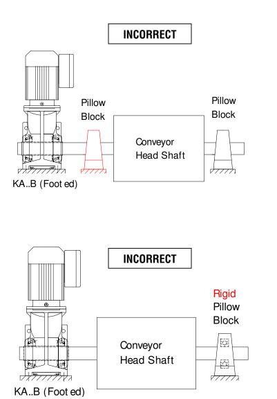
**Problem:** There are four bearings that must be critically aligned. The closer the pillow block bearing is to the reducer, the more critical is the alignment.
