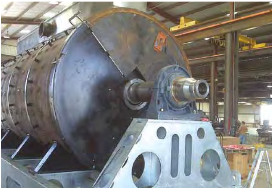
The above 01 series 12-inch Cooper split roller bearing is mounted on a rotating drum that passes steam through a hollow shaft. Due to the intense heat, a C5 clearance bearing along with a bronze roller cage and a special race design allow for 1 3/16-inch of shaft expansion.
