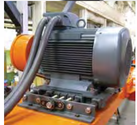
Automatic motor bases can significantly reduce maintenance hours.
