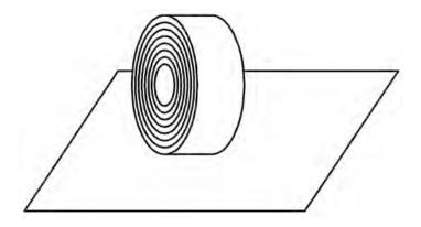
Do not use Storage Method 3 for full or wide rolls of material. It is only appropriate for narrow rolls of belt, and as with Storage Method 2, a pallet or other elevated surface should be used.
