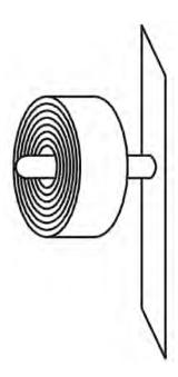
Storage Method 2 is also an effective way of storing material. By storing the belt upright, both edges are equally exposed to the surrounding environment. Belting stored this way should, however, be placed on a pallet or other elevated surface (not directly on the floor) and wound tightly (on a 6.5" OD heavy cardboard or wooden core) to avoid deformation.
