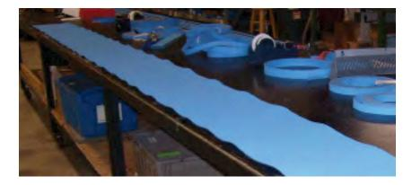
"Abnormal Stresses within Material are Released when Belt is Slit, Resulting in Camber"
