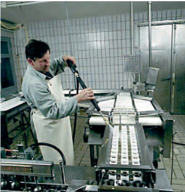
Low pressure cleaning of food conveyor belts
