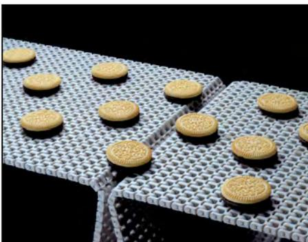
Many food manufacturers embrace the use of plastic modular belts for their sanitary benefits (e.g., non-porous thermoplastics, contoured easy to clean surfaces, partially exposed hinge rods, etc.), low maintenance and ease of repair. Industrial manufacturers also see the value that plastic modular belts add to the bottom line. These inherent benefits include higher strength, lower weight, lower product-to-belt friction levels, as
