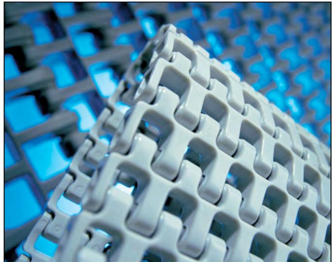
Plastic Modular conveyor belts are assembled in a bricklaid pattern for strength and can be custom-made in virtually any width or length required. Various pitch sizes are also available to support specific conveyor designs-- $\frac{1}{2}$ " pitch belts are used for tight transfers while larger pitch products such as 2" are used to convey heavier loads.
