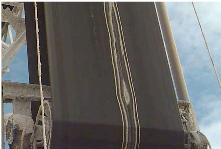
The second and more aggressive type of abrasion is cutting and gouging where jagged or sharp surfaces from materials like limestone, granite, and ores will cut the belt cover and remove the cover in “chunks”. Typical appearance of the surface is shown below.
