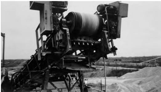
(A head pulley scraper removes material carryback)
